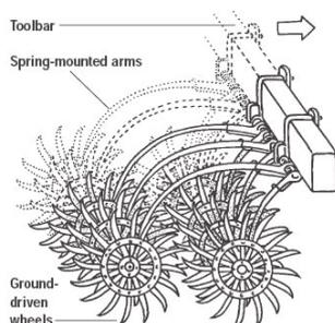
The rotary hoe (Figure 3) referred to in the following section is ground driven, it has one or more sets of vertical star shaped wheels mounted on a horizontal axis. The wheels are 21 inches in diameter with 16 teeth. Speed of work is 15–18 km/hr. They work at 2–3 cm depth. The machine works over the whole field area like the tine weeder.
