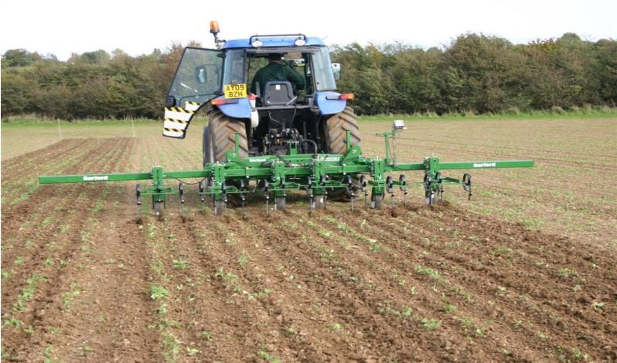
Shows the vision guidance system mounted on Garford's inter-row Robocrop inter-row cultivator. The winter rape was drilled using a GPS controlled drill on 50 cm wide drills.
